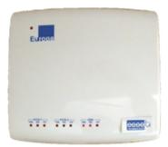
Proprietary modem: allowing for the communication between PC and remote autodialers
