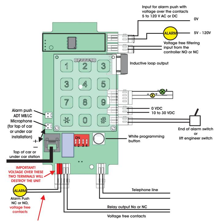
Due to the danger of unwanted induced voltages, the whole length of the cable between the alarm push and this alarm input must be kept away from "voltage cables"
